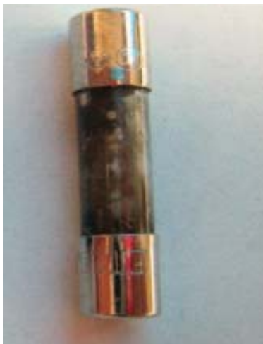
< Fuse, F901 > Can look at physical condition.
