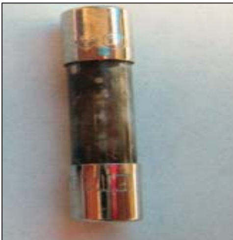
< Fuse, F901 > Can look at physical condition.
